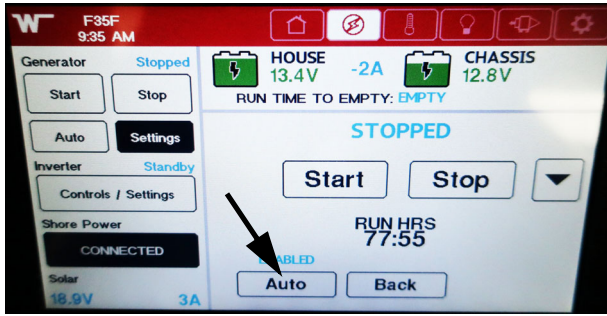
The Auto Operation Condition is displayed as Enabled, Disabled, or Locked out. -Typical View
