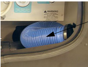
Sewage Drain Hose -Typical View
