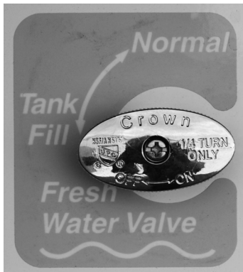
Fresh Water Valve (Located in water service center) -Typical View
